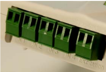
Figure 28: DataNet logger sensor inputs
