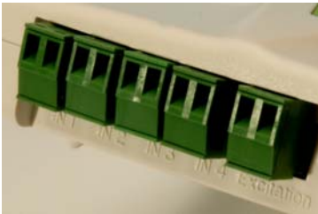
Figure 11: DaqLink logger sensor inputs
